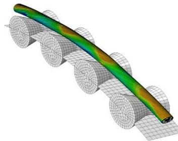
Figure 2: Stress in the umbilical sheave under load
