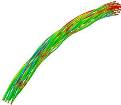
Figure 3: Stress in the tubes under tension
