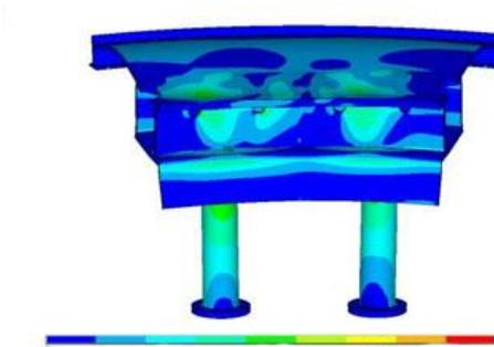
Figure 3: Elastic Stress in the Pedestal Ring under VDE
