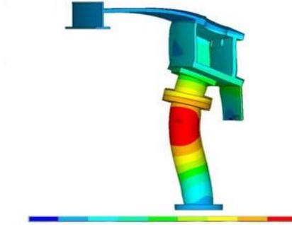
Figure 2: Radial Displacement of Pedestal Ring under seismic loading
