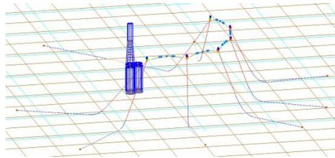
Figure 1: Global set-up of BBRPS 8 point mooring system
