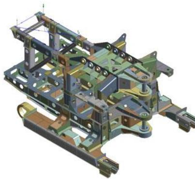
Figure 1: Shell model assembly of mining machine chassis
