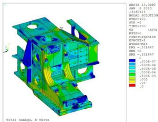
Figure 3: Cumulative damage contour of front track foot
